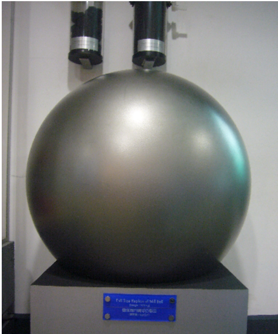
The metal ball used to crush coal granules into powder for combustion
