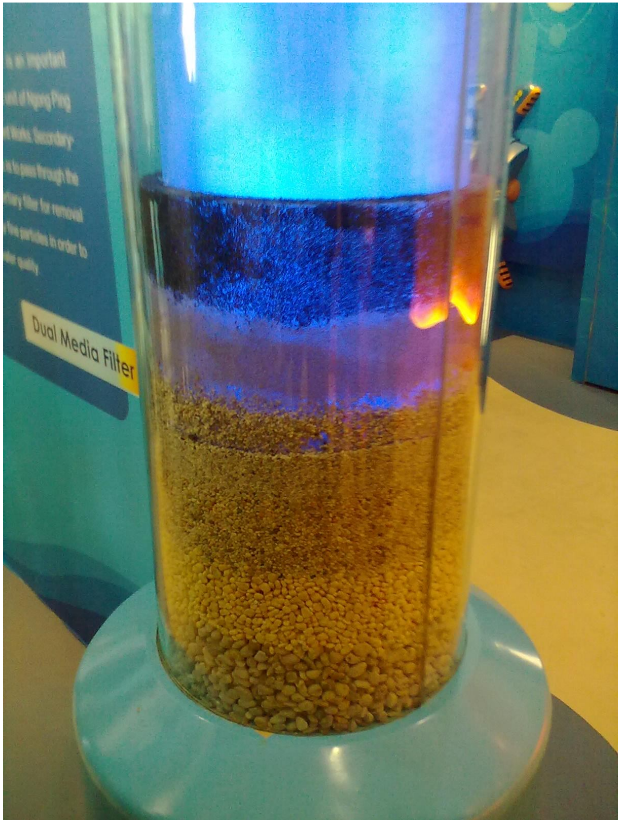
The sewage treatment includes filtration, using activated carbon and clay to remove smell, insoluble impurities. The pebble and sand is used to supply the clay above.
