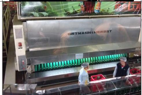
This machine uses in transporting the recycled glass bottles of Coca-Cola. The staff will check whether those bottles are broken so that customers will not get hurt by broken glass.
