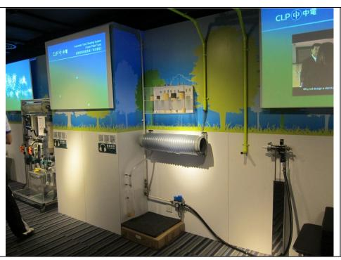
This set-up is showing how to clean the pipes of central air conditioning system used in the large buildings by using a high pressure washer.
