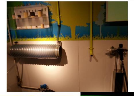
This is a machine which is used to clear to dirty dust in the pipes formed by the air conditioner. It uses very high air pressure to force the stopper to 'walk' along once the pipes it usually used in company which have central air-con system. It is quite interesting.
