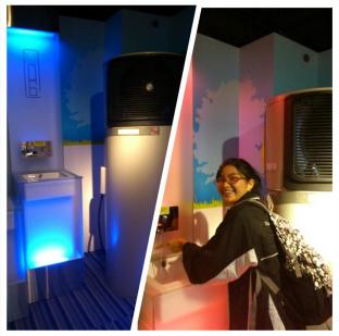
It includes both air-conditioner and geyser. The heat energy produced by the air-conditioner will then heat up the water in the water supply and produce hot water out. This fit in with the principles of "Green Chemistry that it is very energy efficient becaues it will recycle the use of energy before remove them away as a kind of waste.
