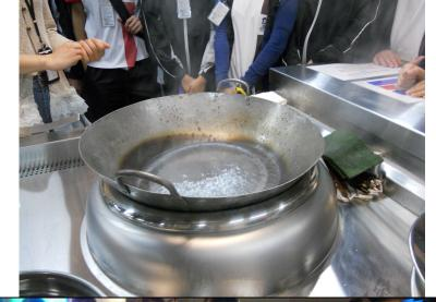
The water in the woke was heated by an induction stove and it boiled in a few seconds only. The heat supplied to the stove was the heat released by the air-conditioning. It increased the energy efficiency and was green.
