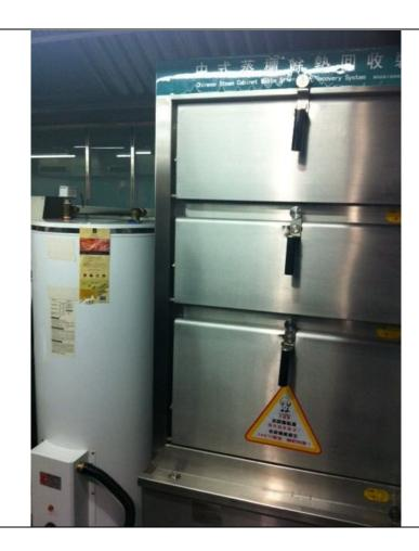
The image shows a Chinese steam cabinet with waste steam recovery system. Extra and unused steam will be passed along the pipes inside the system and for further usage like boiling water. In this way, energy used to form steam is not wasted and the cooking industry can cut cost on energy bills.
