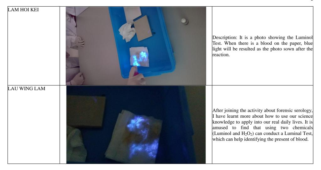
LEONG KA YAU This is a photo of process of the Luminol test. Through this test, we can identify bloodstains from a surface even though the blood is not visible by human eyes. TANG NGAI SIN It is the Kastle-Meyer Test. We add ethanol as an alkaline media, KM reagent and then hydrogen peroxide accordingly. A change in colour from colourless to pink shows the possibility of presence of blood.
