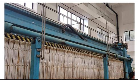
This is the machine that make the dirt to the dirt cakes, it will make the soft dirt change to a piece of dirt cakes.
