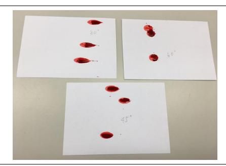
Forensic serology is something new to me. The picture above is a test on how the angle of impact can affect the shape of blood droplet. We can conclude that the smaller the angle of impact, the more the blood droplet to be elongated in shape.
