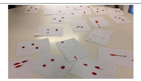
Blood from different heights and different angles will result in different shape! This help to determine the directions and distance of the incident happened.
