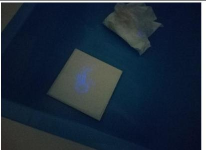
Luminol Test is one kind of blood presumptive testing. First luminal and hydrogen peroxide are added respectively. When blood is detected, we can see shiny blue color appeared.
