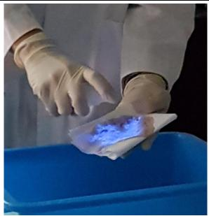
Luminol reacts with iron in haemoglobin, with hydrogen peroxide as catalyst. Blue light can be clearly seen. Luminol test is very useful in crime scene.
