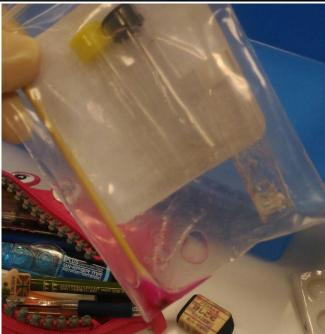
This is the first experiment about indicating if the liquid is blood. The result shown in the photo is a positive one which means the sample tested is blood. The sample is a kind of artificial blood which is pretending to have similar components of organisms' blood. The positive results will show a colour change from green to pink.
