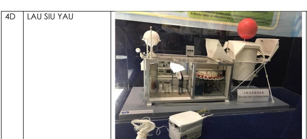
It is an actual model of Automatic Upper-air Sounding System. The radiosonde dangling inside which contains temperature and humidity sensors will measure weather information when the balloon rises.
