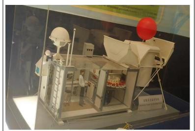
The balloon in the Automatic Upper-air Sounding System rises every 8 a.m. and 8 p.m. at King's Park to observe the pressure, temperature and humidity of upper-air.
