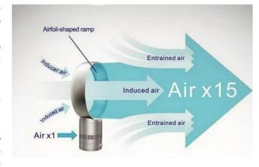
airplane wing bent around into a loop. The air encounters what would be the leading edge of the wing, said Dyson engineer Andy Samways. When it hits the wing-like structure, the air speeds up, creating an area of low pressure.
